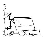
**Important**: After terminating work it is essential that the disc brushes and the brush rollers are relieved of strain (danger of deforming the brushes).
