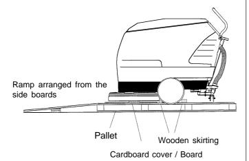
Make a ramp from the long, side boards of the packing by laying them on the pallet. Secure the boards with nails. Lay the shorter boards under the ramp for support. Remove wooden skirting.
